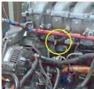
Figure 18: knock sensor correctly placed.
