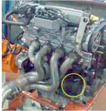
Figure 19: knock sensor incorrectly placed.
